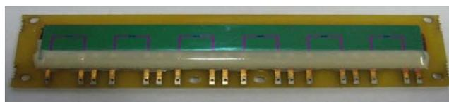
Fig. 3. Photo of 6-channel sensor line on the basis of silicon pH-FETs.
