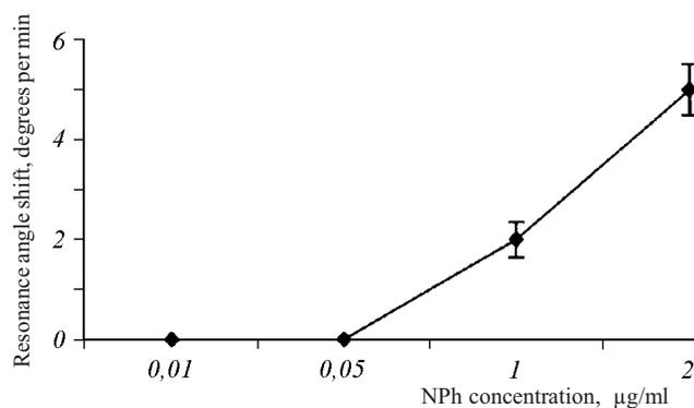
Fig.4 Response of the immune sensor to the introduction of different concentrations of NPh into the measuring cell with preliminary modification of the sensor surface with dextran sulphate and glutaraldehyde
