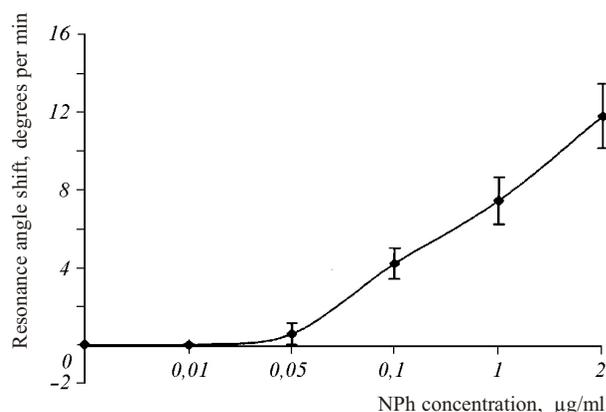
Fig.1 Response of the immune sensor to the introduction of different concentrations of NPh into the measuring cell with non-modified transducer surface
