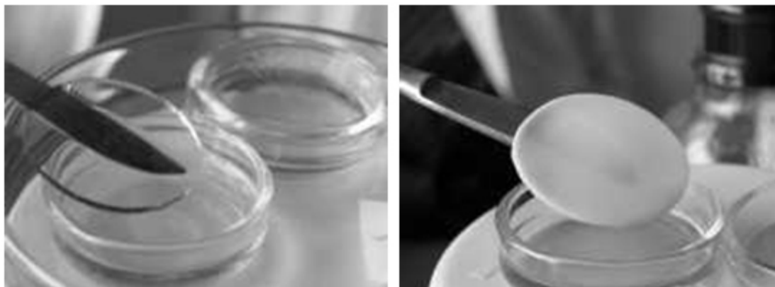
Fig.2. General appearance of hydrogel membranes after swelling in cultivation medium DMEM.
