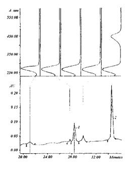
Fig. 3. HPLC profiles of reaction mixture of oligonucleotide labelling with Cyan 39 and absorbance spectra of components: I - 5'-NH<sub>2</sub>- $(CH_2)_6$ -NH-COO-(Tp) 1 4T; 2 - 5'-Dye- $(CH_2)_6$ -NH-COO-(Tp)<sub>14</sub>T ( $^{abs}$  $\chi_{max}$  446 nm)
