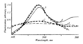
Fig. 4. Fluorescence spectra of free Cyan 40: I = 5'-Dye- $(CH_2)_6$ -NH-COO- $(Tp)_{14}$ T; 2 — and duplexes of oligonucleotide-dye conjugate with poly(dA) (3) and poly(rA) (4)
