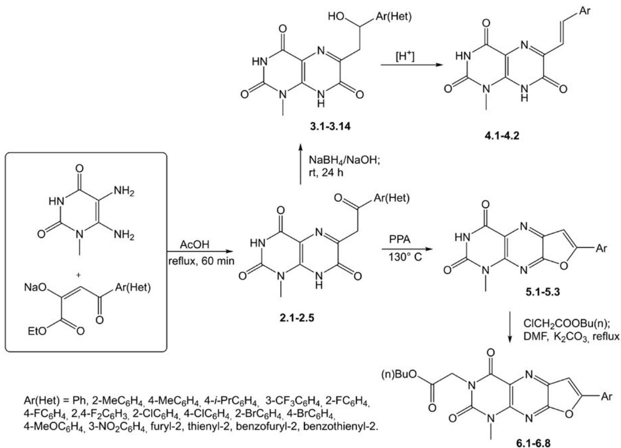
**Fig. 1.** Synthesis of 6-substituted 1-methylpteridine-2,4,7-triones (**2.1–2.5**, **3.1–3.14**, **4.1–4.2**), 1-methyl-7-arylfuro[3,2-g]pteridine-2,4(1*H*,3*H*)-diones (**5.1–5.3**) and butyl 2-(1-methyl-2,4-dioxo-7-aryl-1,4-dihydrofuro[3,2-g]pteridine-3(2*H*)-yl)acetates (**6.1–6.8**)
